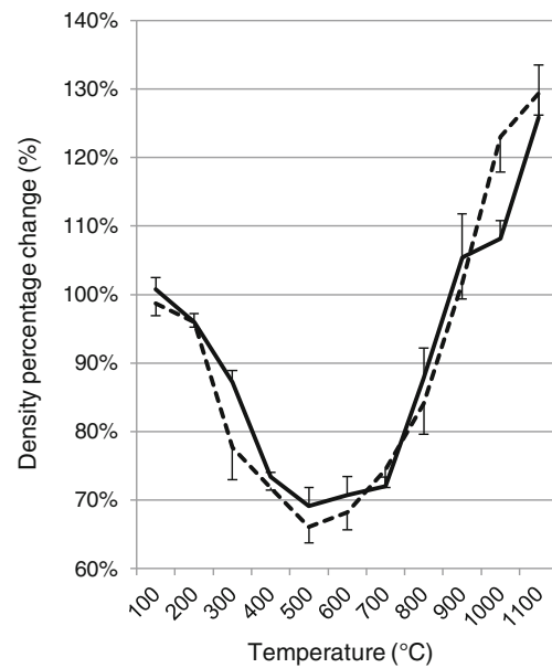
Fig. 3 Changes in density calculated from values obtained for the weight and volume analyses in Fig. 1. Data are the percent density change with respect to values before burning (indicated as 100 %). Specimens were burnt for 30 min (solid line) or 2 h (dashed line). Error bars indicate the standard deviation ( n=3 )
